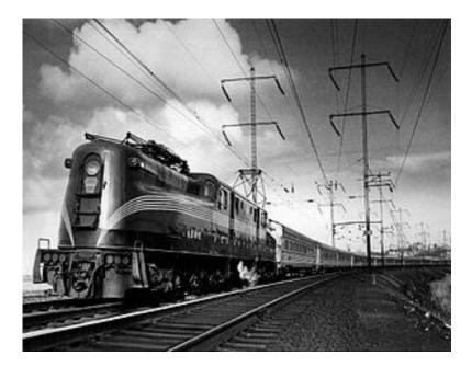
Act 89 of December 18, 1987, designated the Pennsylvania Railroad GG1 4859 Electric Locomotive as Pennsylvania's official electric locomotive. The locomotive was built in 1937 in Altoona, Pennsylvania. The high-speed engine powered passenger trains, troop trains in WWII, coal, and freight.
