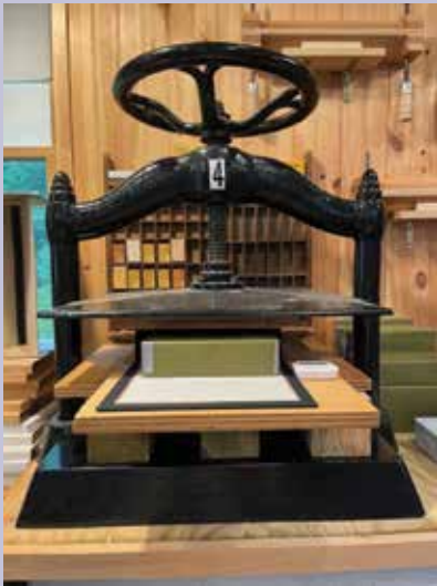
Above: A press like this is used to ensure the glued surfaces are solidly attached.
